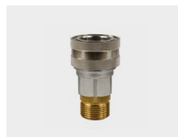
Coupling : M. Nickel-plated brass + brass. Max. 250 bar / 150 °C
