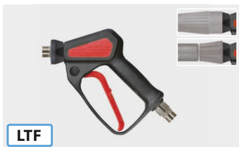
Professional ultra high pressure gun with patented LTF. Gun with insulated outlet suitable for lances with swivel screw coupling. Max. 500 bar / 30 l/min / 150 °C
