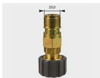
Plug : F. Zinc-plated steel + brass. Max. 250 bar / 150 °C
